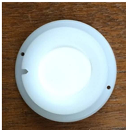
Figure 1. Actual device showing plastic body and filter actual size is 2.5 cm or 1 inch (Left). Note gel is below the filter. Drawing with components (right).
